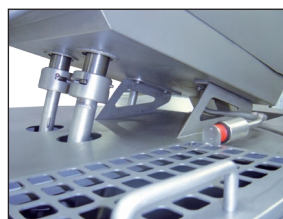
Clamping device for the scraper arm and satellite.
