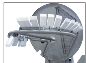
Inclined, removable scraper arm and satellite mixer.
