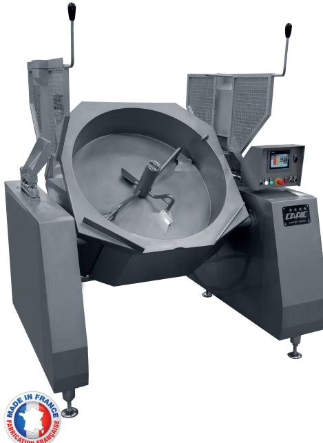
The height of the tank is 295mm, in order to respect the final aspect and organoleptic qualities of products.
