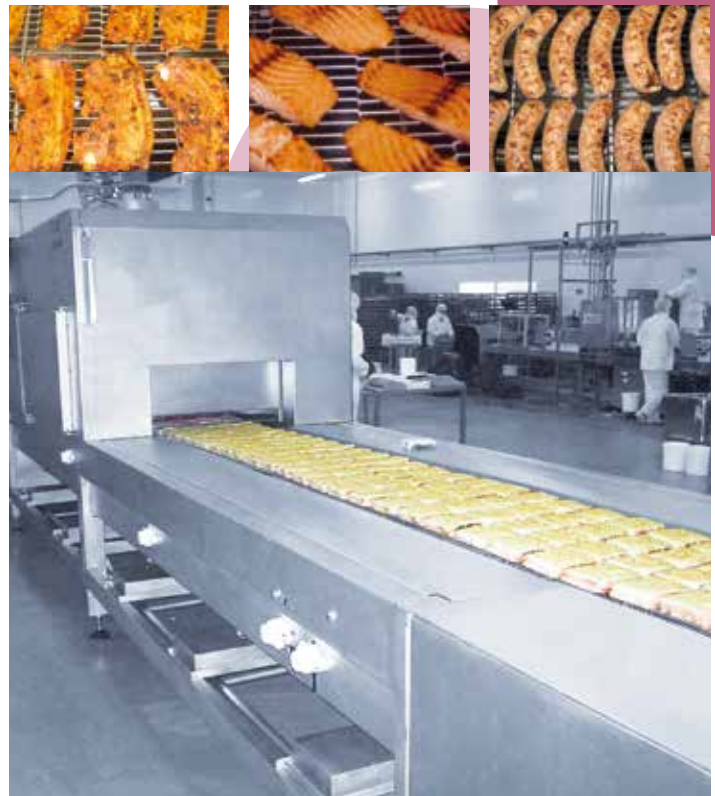
Radiant heating on 3 sides.
