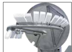
Inclined, removable scraper arm and satellite mixer.
